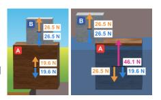
it is in the pool. When the blocks are on the ground, this contact force is not present (left scenario).
