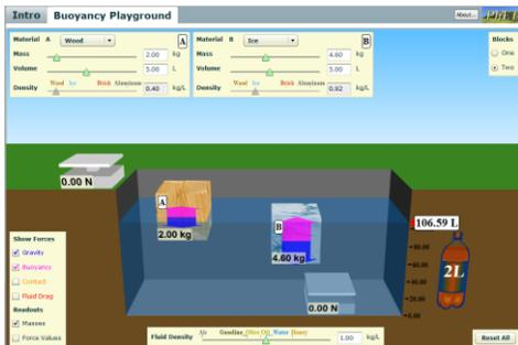
**Buoyancy:** When will objects float and when will they sink? Learn how buoyancy works with blocks. Arrows show the applied forces, and you can modify the properties of the blocks and the fluid.
