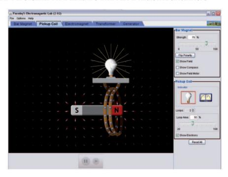
Fig. 5. – Screenshot of Faraday's Electromagnetic Lab. Here the "Pick up Coil" tab is shown when the magnet is moving to the right through the coil. The red and white diamonds represent the magnetic field and the blue spheres represent electrons.
