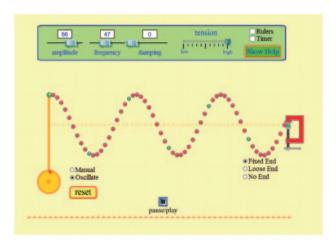
Fig. 3. – Wave on a String simulation. The user can grab the end of the string and oscillate it or use the oscillator to do it for them. Amplitude, frequency, damping, tension and time are all adjustable.
