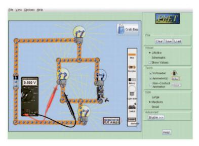
Fig. 4. – The Circuit Construction Kit (CCK). This simulation allows users to build any circuit they can imagine with wires, batteries, resistors, light bulbs and switches. An ammeter and voltmeter are available for taking measurements. When a circuit is completed the electrons move and the light bulbs will light!
